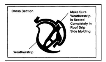
5. Using finger pressure, press the length of the weatherstrip between the No. 1 and No. 3 corners to verify that the weatherstrip is seated completely in the roof drip side molding as shown in illustration.
