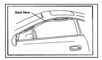
2. If the weatherstrip is in good condition, start by installing the weatherstrip in the No. 2 corner. If the weatherstrip is damaged, replace the weatherstrip.
