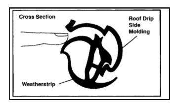
3. Hook the bottom edge of the weatherstrip into the roof drip side molding first. Then, using your fingers, install the top edge of the weatherstrip into the molding.
