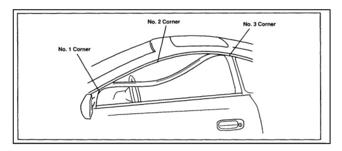
The installation method of the roof side rail weatherstrip has been modified to improve retention between the No. 1 and No. 3 corners on 2000 model year Celica vehicles. The part has not been changed. Use the following installation instructions to reinstall the roof side rail weatherstrip on vehicles with the above concern.
