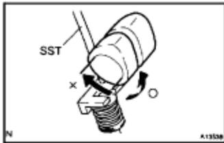
(5) Rotate the crankshaft so that the camshaft is positioned as shown in the illustration.
