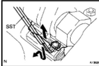
(b) Remove the adjusting shim.
