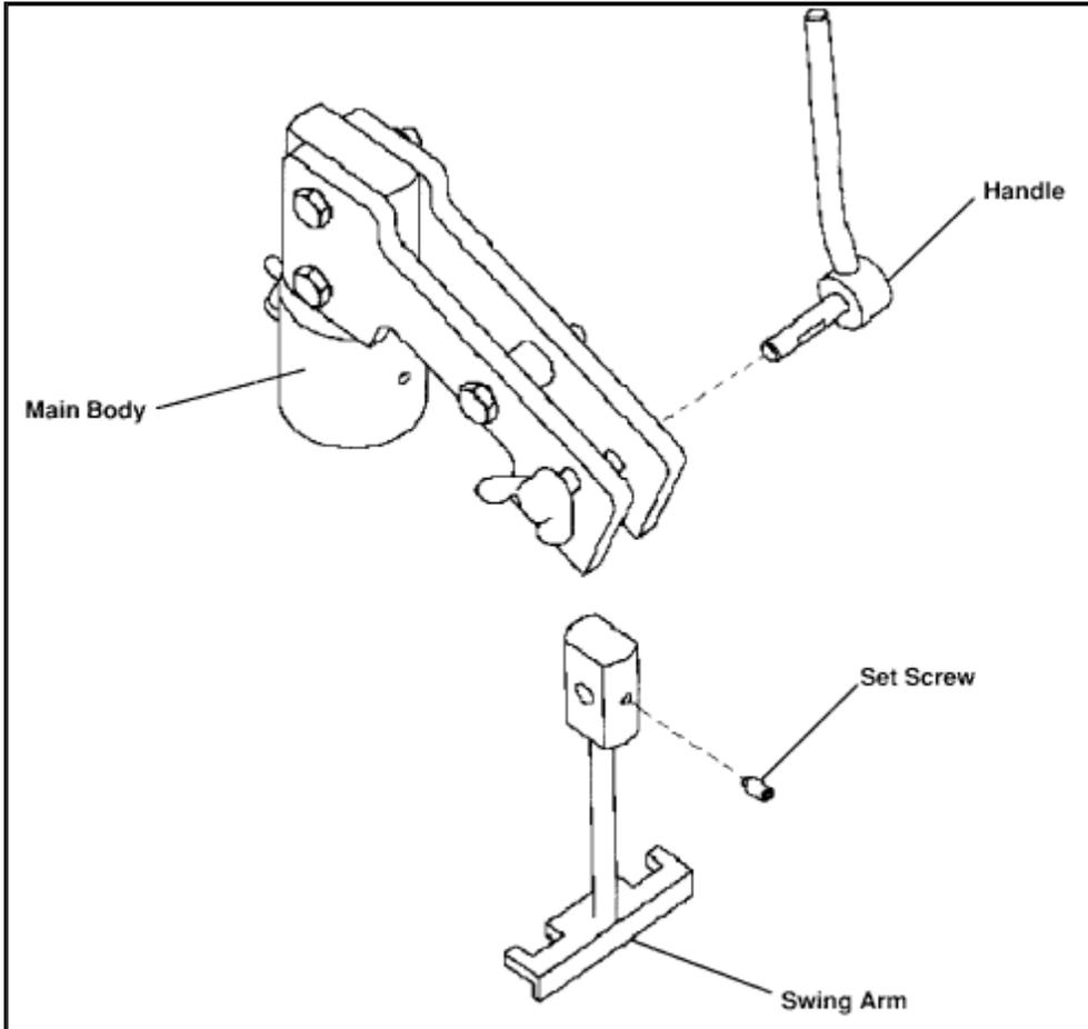
1. Remove the 2 mm set screw from the swing arm using the Hex wrench supplied.
