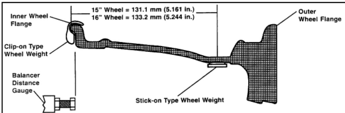
1. Mount tire/[wheel](#) assembly on wheel balancer with the outside or decorative wheel flange opposite the wheel balancer arbor.
