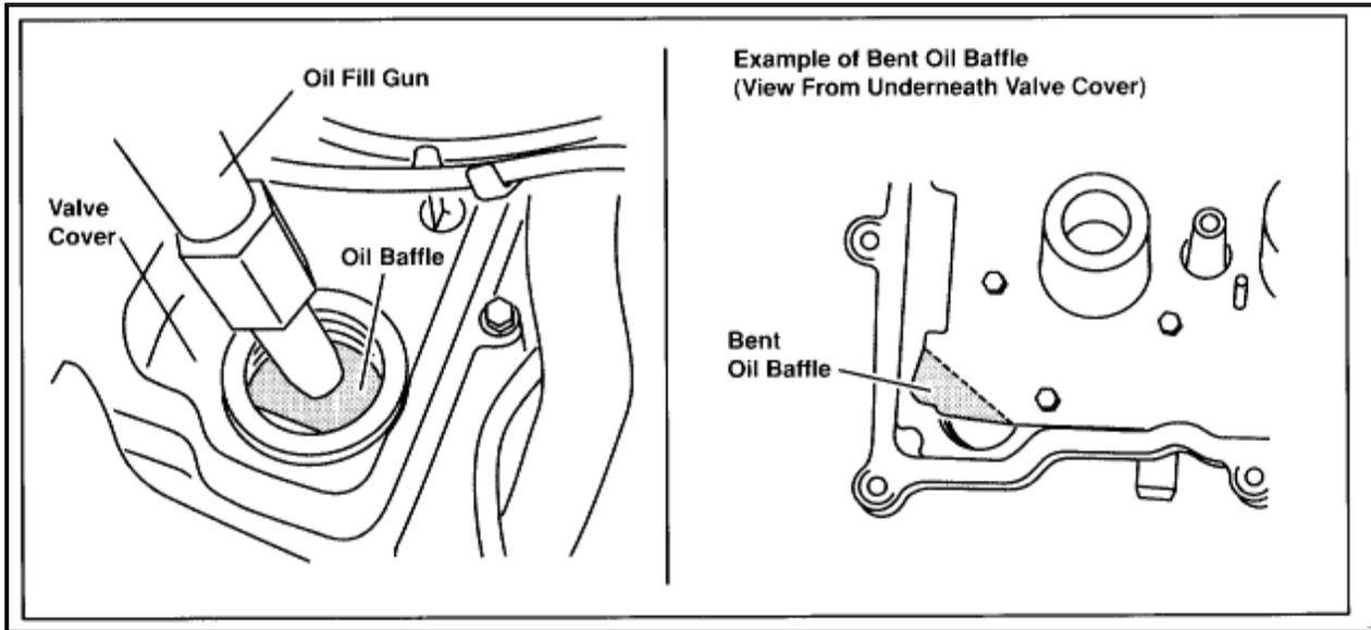
To help prevent unnecessary complications during the oil fill process, no undue load should be placed on the oil baffle attached to the inside of the [valve cover](#) (see illustration). This baffle is designed to deflect oil and should not be used to support the weight of heavy oil fill devices. These devices can place stress on the baffle, and bend or break it during the oil fill process.
