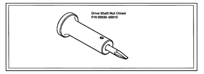
The function of the Drive Shaft Nut Chisel is to properly bend the detented portion of a locking nut out of the way of shaft threads for removal of the nut. This is important to eliminate the possibility of thread damage during nut removal. After nut installation, the tool can also be used to stake the locking nut.
