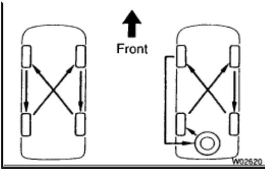
**HINT:** See the illustration for where to rotate each tire when you include the spare tire in the rotation and when you do not.
