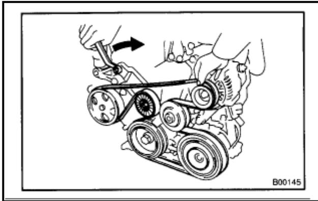
1. REMOVE DRIVE BELT Turn the drive belt tensioner slowly clockwise and loosen it. Then, remove the drive belt and replace the drive belt tensioner little by little and fix it quietly.
