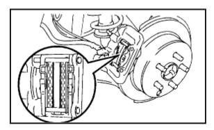
2. INSPECT PAD LINING THICKNESS Check the pad thickness. Minimum thickness: 1.0 mm (0.039 inch)
