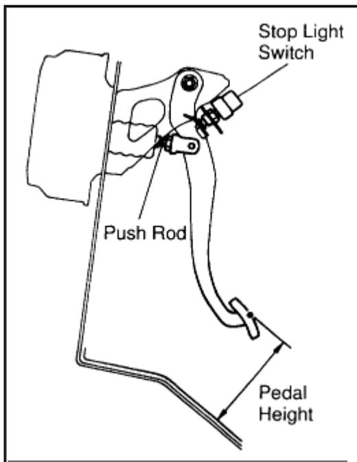
1. CHECK PEDAL HEIGHT Pedal height from asphalt sheet: **139.8 - 149.8 mm (5.504 - 5.898 inch)** If the pedal height is incorrect, adjust it.
