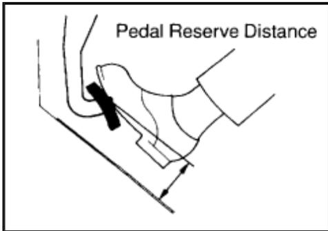
4. CHECK PEDAL RESERVE DISTANCE Release the [parking brake lever](#). With engine running, depress the pedal and measure the pedal reserve distance, as shown. Pedal reserve distance from asphalt sheet at **490 N (50 kgf, 110.2 lbs)** : **More than 85 mm (3.35 inch)** If incorrect, troubleshoot the brake system.
