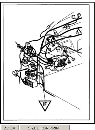
E. Properly attach and route the new wire to the exterior of the existing wire harness in a manner that will not allow it to become damaged or come into contact with any other circuits.
