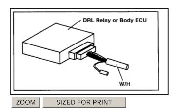
2. Use the locking pick tool from the wire harness repair kit and back out the terminal from the appropriate connector for the DRL Relay or Body ECU. See the Reference Chart as shown in this bulletin for pin and connector information.
