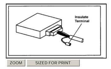
3. Insulate the removed terminal using vinyl electrical tape.
