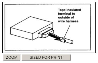
4. Secure the wire and terminal to the outside of the wire harness using vinyl electrical tape.
